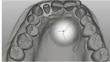
8. Upon design approval, the Atlantis Abutment Core File is provided allowing to start CAD design of the provisional crown.
